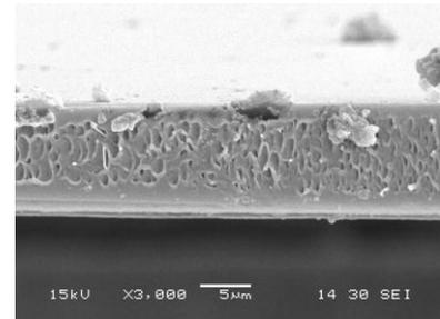
Figure 4: SEM analysis of sericin film (PVA+Gly+S<sub>R</sub>)
