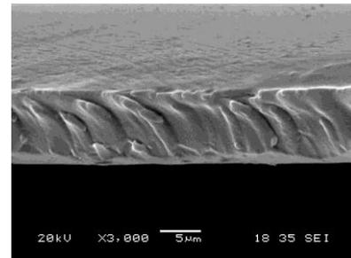
Figure 3: SEM analysis of pure PVA film
