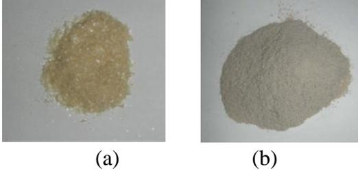
Figure 1: Powder sericin; (a) commercial (b) recovered from wastewater.
